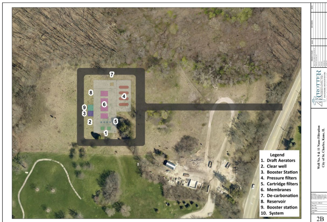
Figure 6-4: Well #9/11 Reverse Osmosis Treatment Facility
