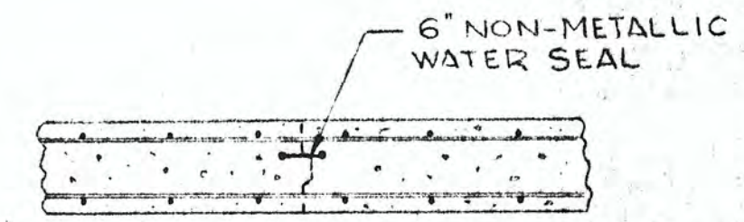
TYPICAL WALL CONSTRUCTION JOINT
