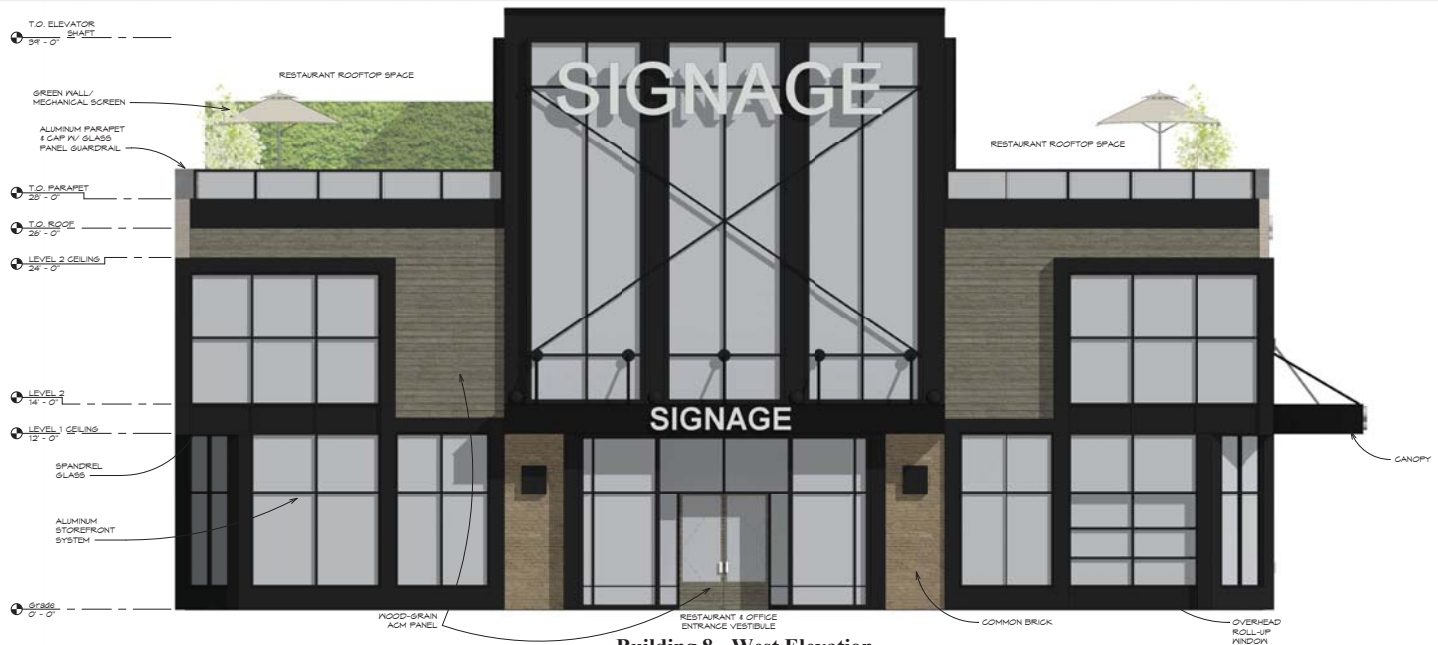
Building 8 - West Elevation Scale: 1/4" = 1'-0" SOUTH 2nd STREET
