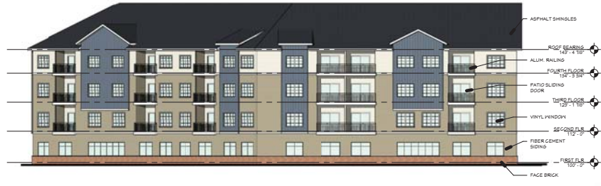
3 EAST ELEVATION PR-3.2 1/16" = 1'-0"
