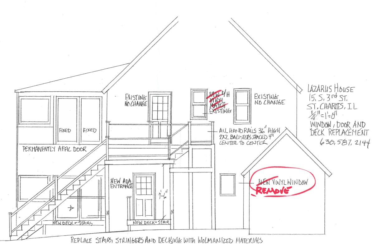
REPLACE STAIR, STRINGERS AND DECKING WITH WOLMANIZED MATERIALS AUL RAILS TO BE 36" HIGH WITH 4" SPACED 2X2" BALISTERS EXISTING 6"X6" COLUMNS TO REMAIN ON FROST PROTECTED PIERS
