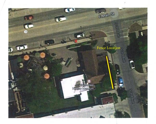
The fence is to have 6-7 brick posts and be 52 feet long. The posts should be about 3 feet tall and be 20-20 with another foot on top for flowers. The fence will be 1 foot in from the east sidewalk.
