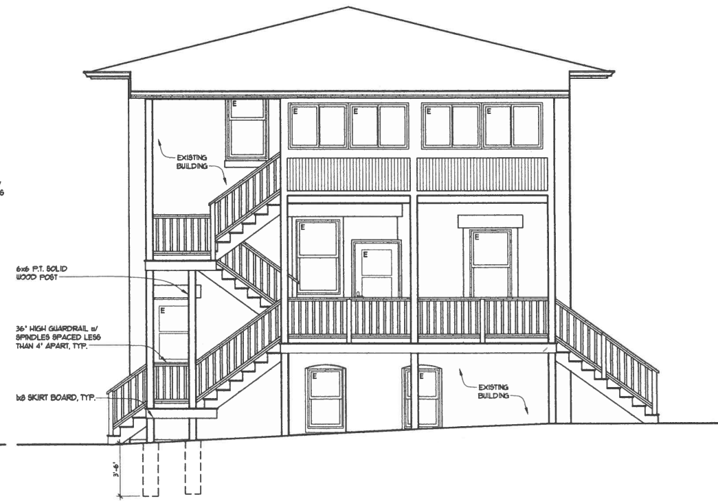
NORTH ELEVATION E • EXISTING SCALE: 1/4" = 1'-0"
