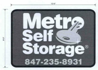
(2) COMPLETE S/F INTERNALLY ILLUMINATED CABINET SIGN WITH FLEX FACE. FIRST SURFACE VINYL DECORATION, THE CABINET IS TO HAVE RADIUS CORNERS. THE RETAINER IS FIGURED FOR 4". THE CABINET DEPTH IS TO BE 1'-6". THE SIGNS ARE TO BE FLUSH MOUNTED TO WALL. FLUORESCENT LAMP ILLUMINATION. THE SIGN IS TO BE UL LISTED WITH A SERVICE SWITCH INSTALLED.
