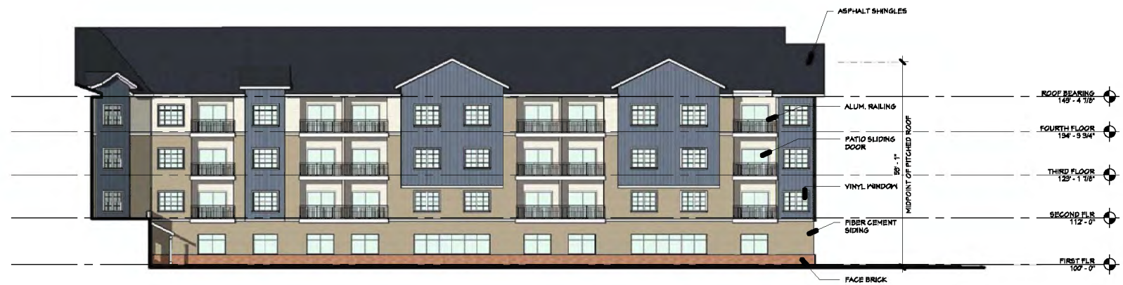
1 NORTH ELEVATION PR-3.2 1/16" = 1'-0"
