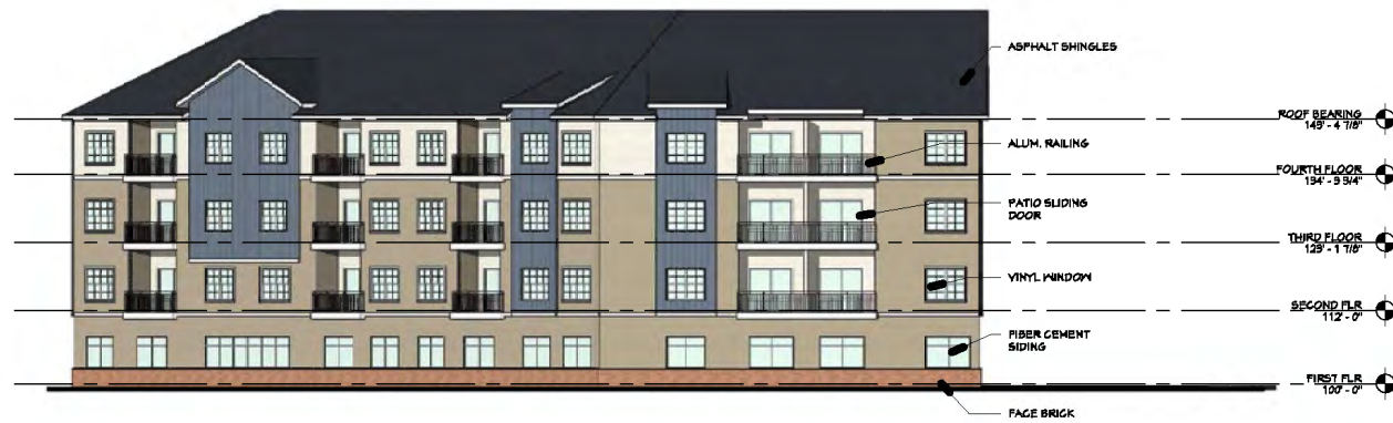
3 EAST ELEVATION PR-3.2 1/16" = 1'-0"
