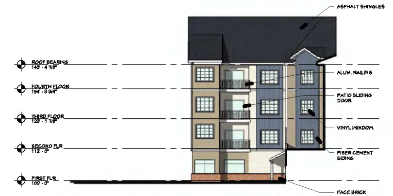
5 WEST ELEVATION PR-3.2 1/16" = 1'-0"
