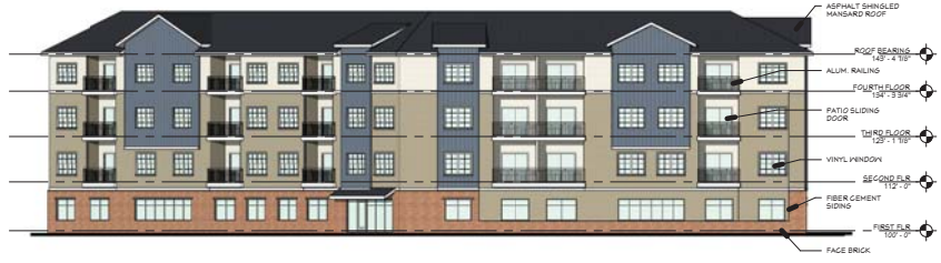
3 EAST ELEVATION PR-3.2 1/16" = 1'-0"
