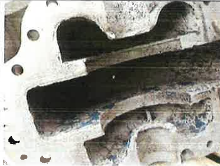
Heavy pitting on interior of castings
