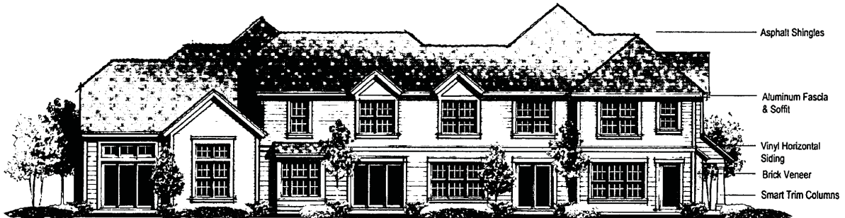
Rear Elevation - 4 Unit Building scale: 3/16" = 1'-0"
