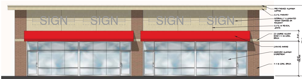
1 SOUTH ELEVATION (FACING LINCOLN HWY/ RTE 38) SCALE: 1/4" = 1'-0"
