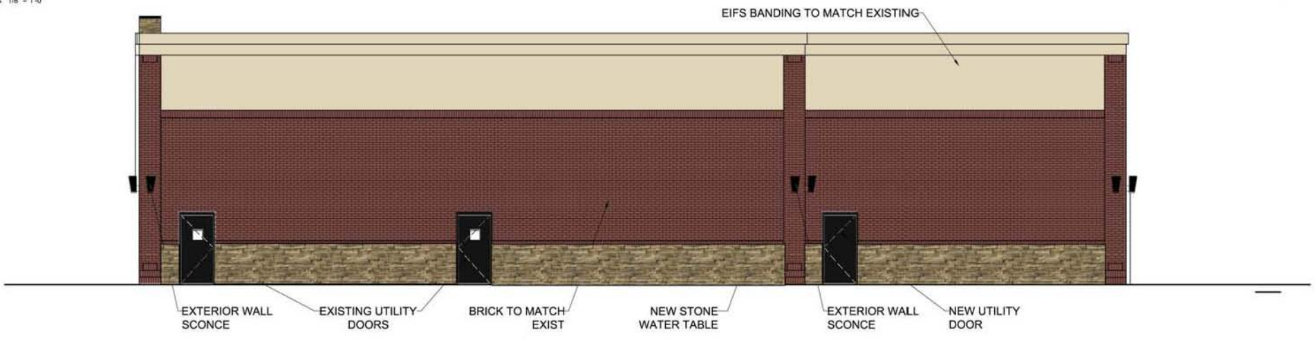
1 PROPOSED SOUTH ELEVATION SCALE: 1/8" = 1'-0"
