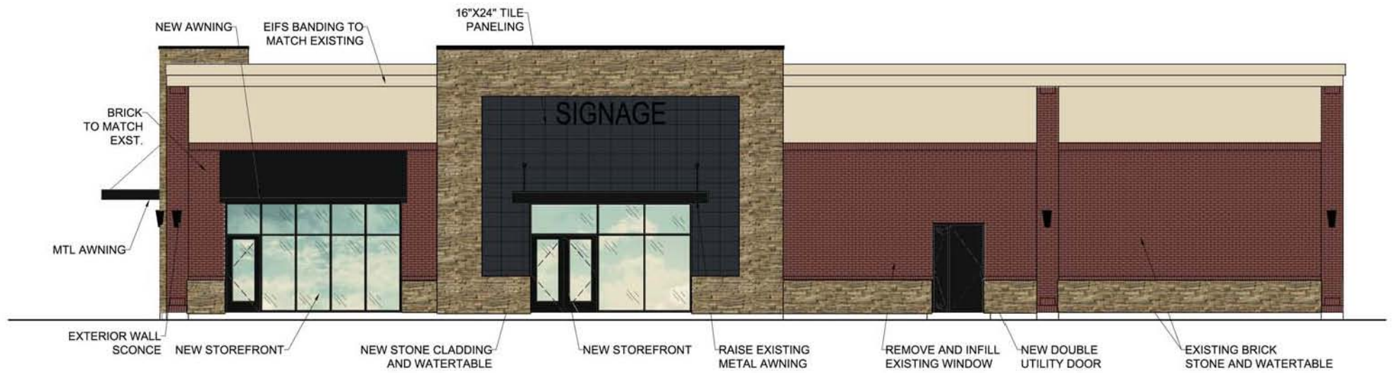
2 PROPOSED WEST ELEVATION SCALE: 1/8" = 1'-0"
