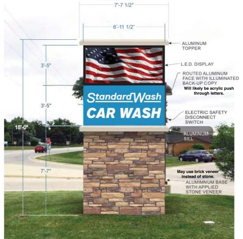
A SOUTHEAST ELEVATION - WITH INTERNALLY ILLUMINATED DOUBLE-FACED MONUMENT VERSION 1 (NOTE: THIS SIGN IS IDENTICAL ON BOTH SIDES). SCALE: 3/8" = 1'-0"
